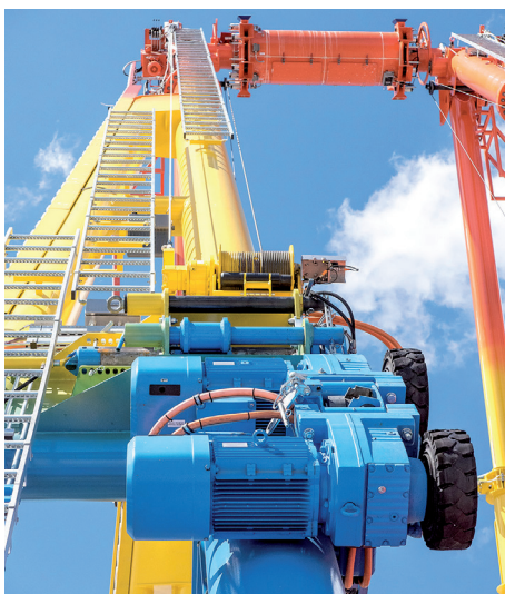
Fig. 4: A total of eight energy-efficient helical gearmotors with a nominal power rating of 18.5 kW drive the giant wheel via pairs of friction wheels.
