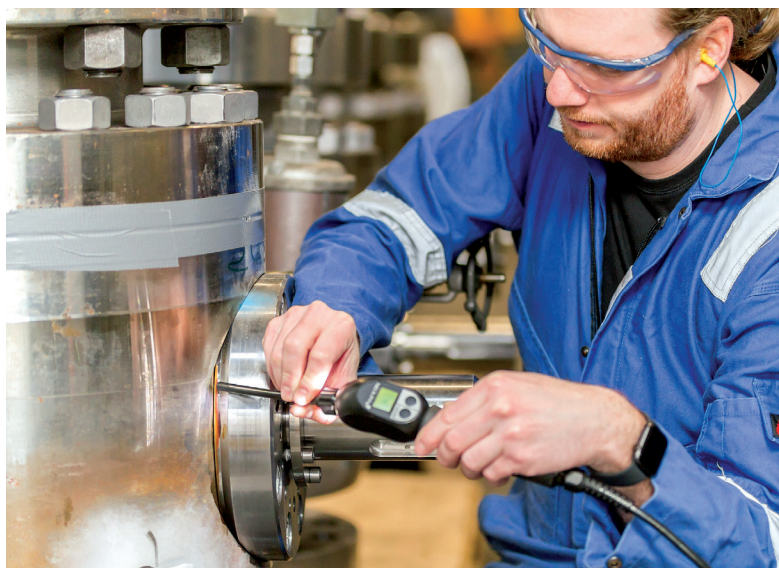
A pressure test with hydrogen shows whether the limit values are complied with and fugitive emissions are minimised. Photo: Hartmann Valves
