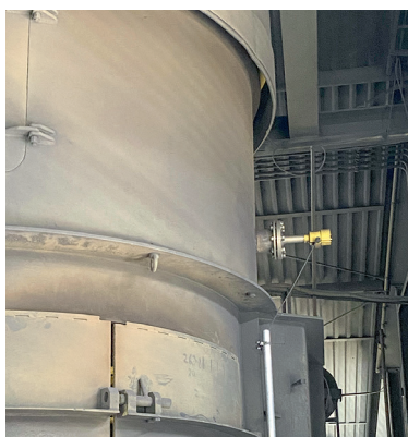
Fig. 3: The conditions around the shaft furnace are harsh. However, the radar sensors are not impressed by dust or the high temperatures.
