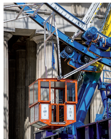
Fig. 3: Special v-shaped gondola hanging arms allow each of the gondolas to hang more freely and give every passenger an unobstructed view. The enclosed design of the gondolas also makes them especially suitable for younger passengers.
