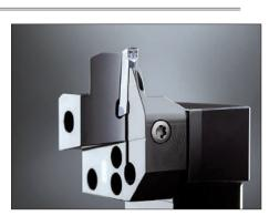
To accommodate axial grooving operations with diameters ranging from 38 mm to 1,000 mm, Horn is now offering new holder variants for the S224 grooving system
