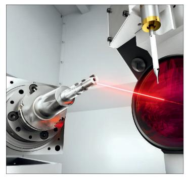
The VOLLMER VLaser 270 machine's laser light and innovative kinematics ensure the fast and high-precision machining of tools with ultra-hard cutting materials
