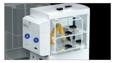
Robot loader with the externally installed tool cleaning (1) and laser marking modules (2)
