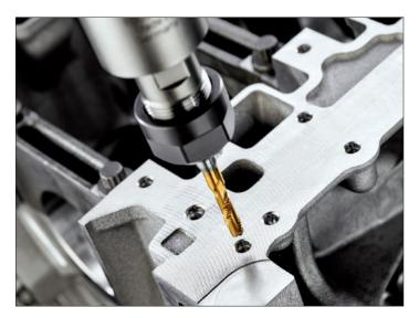
*The Punch Tap technology enables internal thread production in a quarter of the time*
