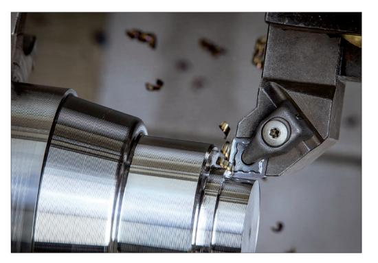
For the machining of steel, stainless steel, superalloys and non-ferrous metals users only need the multi-application grades CTPX710 or CTPX715 from CERATIZIT
