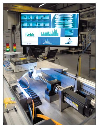
System developed at KIT for fully automatic wear control of ball screws by using artificial intelligence photo: Markus Breig, KIT
