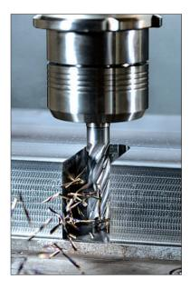
The CCR milling cutters are ideal for trochoidal milling strategies and enable an extremely high chip volume
