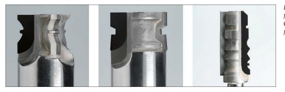
Laser processed PCD tools for eyewear industry in a  $\emptyset$  range of d = 4 - 8 mmfor cutting lenses
