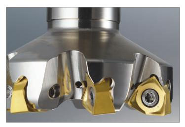
forces and together with an increase in insert thickness compared to conventional types, also provides excellent resistance to breakage. Furthermore, a high maximum depth of cut of up to 8.2 mm enables efficient shoulder milling capabilities. In order to meet component surface finish expectations, the bottom of all inserts feature a large radius geometry that acts like a traditional wiper.
