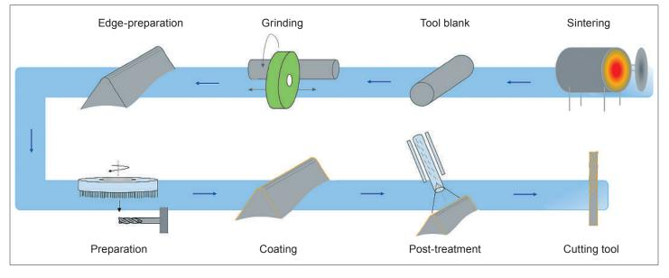
figure 1 Steps of the cutting tool manufacturing [Fraunhofer IPA]
