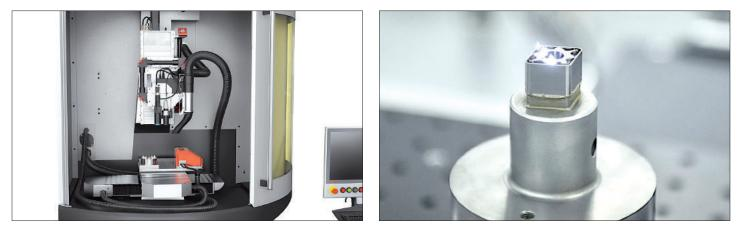
The femtosecond laser emits light pulses, the duration of such a pulse is in the femtosecond range (1 fs = 10-15 sec.), its power is 20 W; with laser ablation, hardly any heat is brought into the workpiece and almost any material can be processed
