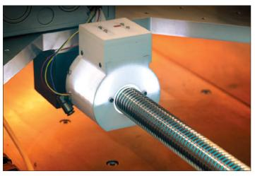
An integrated camera with lighting enables continuous monitoring of the spindle in the ball screw drive photo: Markus Breig, KIT
