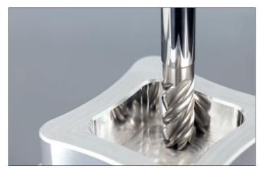
*The patented Franken Cut&Form end mill enables finishing and polishing of the workpiece in one operation*
