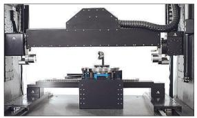
The sensor bridge is configurable, allowing the most optimal and appropriate sensor selections to suit the part and surfaces, in addition to the complex dimensions being measured
