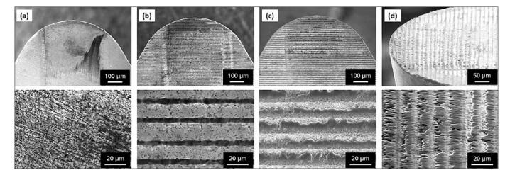
figure 4: Miroscopic images of tools with different rake face structuring<sup>[19]</sup>
