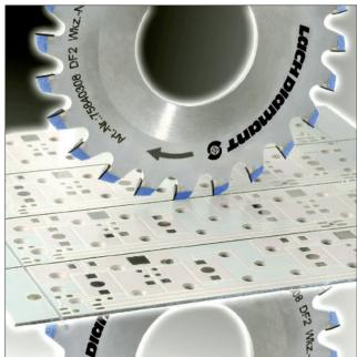
LACH DIAMANT "DreboBlueCut" scoring saw development status as of 2018 -"World Running Champion" not only during PCB machining but also (as shown in photo) during the scoring of aluminium IMS circuit boards
