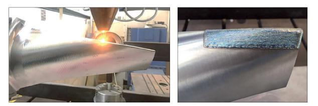
Repairing a turbine blade using laser deposition welding; images: CHIRON
