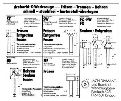
Excerpt from catalogue "Trennen, Fräsen, Entgraten, Bohren von GFK, Duroplasten und anderen Werkstoffen mit PKD-Werkzeugen", published on the occasion of productronica 1977 - in the beginning, the schematically shown shank tools could only be fitted with segments from approx. Ø 3.4 mm circular blanks
