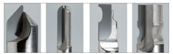
Laser processed PCD tools for eyewear industry in a Ø range of d = 6 - 8 mm
