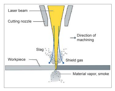
figure 2 Schematic of laser machining [Trumpf]
