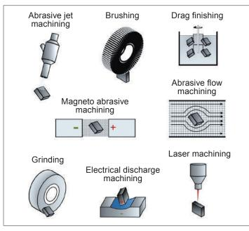
figure 3 Methods for cutting edge preparation<sup>[13]</sup>
