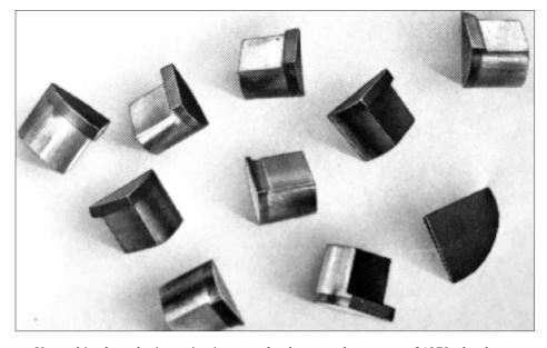
Unmachined synthetic cutting inserts - developmental status as of 1973; the shown segments with 60° and 90° angles were mechanically cut out of PCD blanks (of approx. Ø 3.4 mm) with diamond cutting wheels
