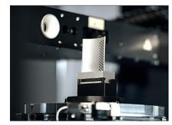
The sensors can be configured to the specific GD&T measurements and the part, and in one scan can capture data points to create a high-density 3D model
