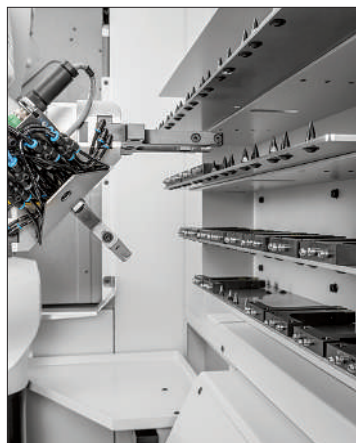
RS05-2 robot system – change of finger grippers – high clamping range for a wide range of workpiece dimensions
