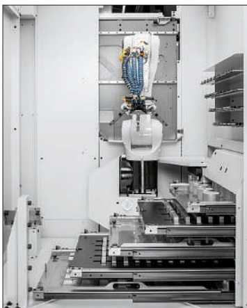
RS05-2 robot system – 5-fold drawer storage with universal dies for individual and large workpiece storage
