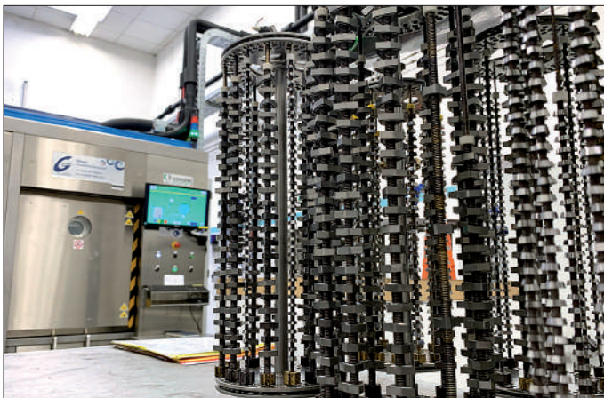
Broad innovation and investment offensive at Boehlerit: the new cleaning system optimally prepares the inserts for coating (photo: Boehlerit)
