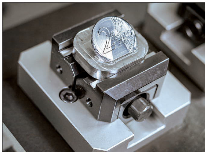
Extremely small but incredibly strong: the ZSG mini from the WNT performance range by CERATIZIT is the ideal partner for clamping small workpieces
