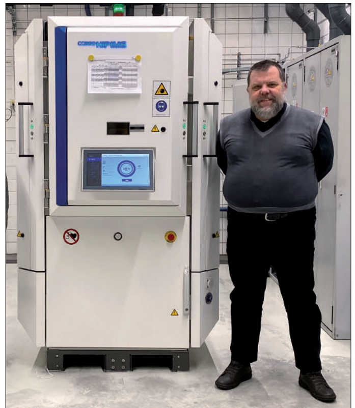
Dr Arno Köpf next to the CC800® HiPIMS from Boehlerit: "In the past, PVD was considered for milling, CVD for turning. The HiPIMS technology changes this abruptly.
